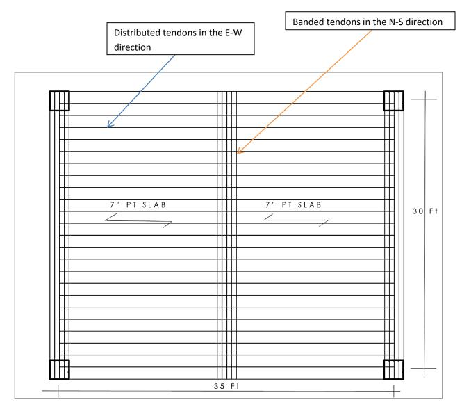
Figure 18 post-Tension tendon layout
