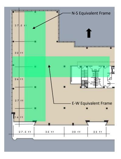
Figure 19 Equivalent frames chosen for PT design highlighted in green
